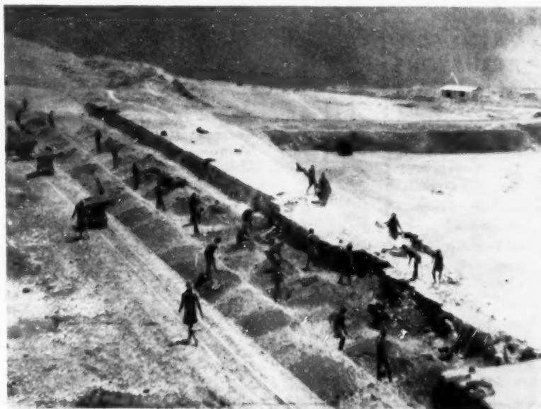
At Rutongo, Ruanda the Bahutu tribesmen dig and load cassiterite bearing gravel which is transported to washing plants in the two ton rocker bottom cars.
